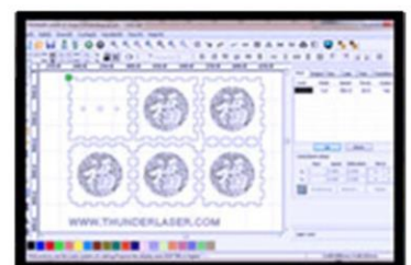
Color mapping Change the working speeds and power by using color settings.
